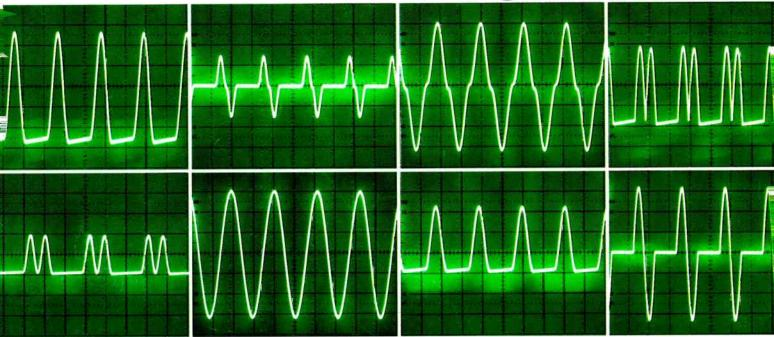
The new TX81Z is the first FM tone generator from Yamaha that offers eight different waveforms for each operator. So besides sine waves, now there are seven other exciting waveforms you can play with.
