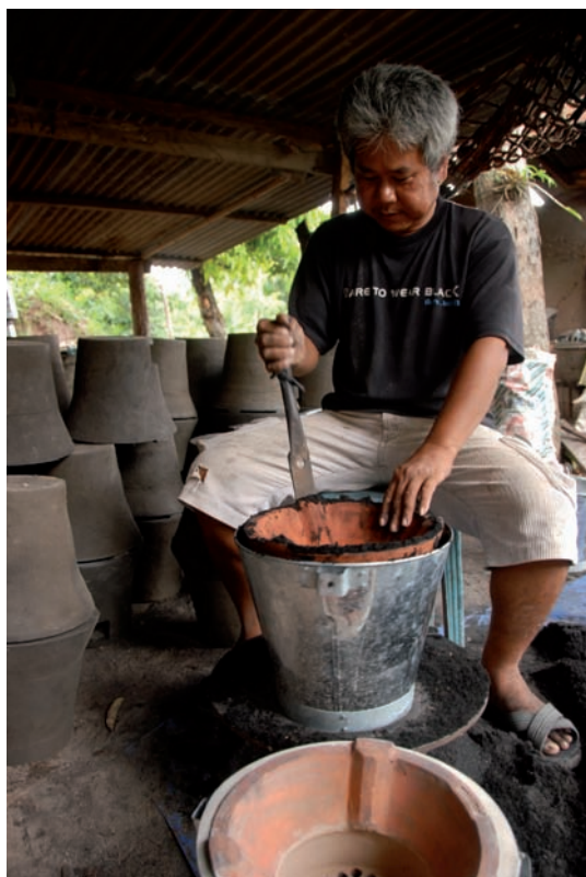
Boonchoo is placing a mixture of rice husk and soil in a stove as heat insulator.
