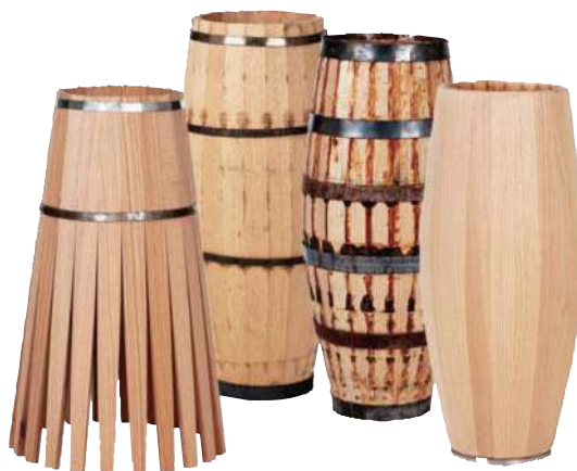
The birth of a conga, from strips of red oak to assembled shell
