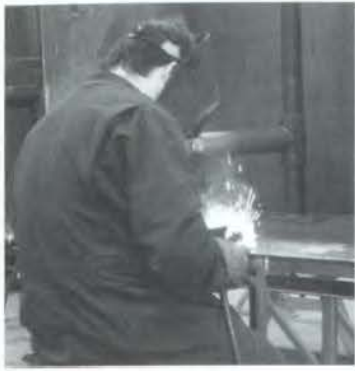
A weld in progress, sophomore Shon Ebbs does a Mig Tee weld. "I took two pieces of metal and tacked them to look like a 'T' then I used a Mig machine and welded three passes on each side," explained Ebbs.
