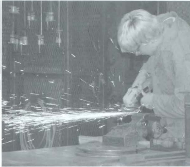
Let the sparks fly, senior Joel Delgado grinds a guided bend project where two pieces of metal were welded together, then cut, and bent to test the weld's strength.
