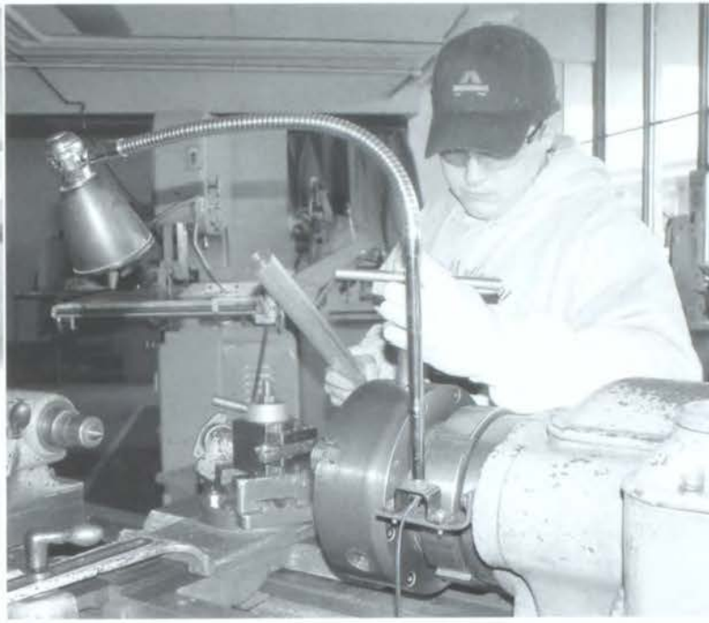
Using the chuck key, sophomore James Barker works to finish his project, a small aluminum bat into which he drilled a hole in the middle and put a brass fitting inside.
