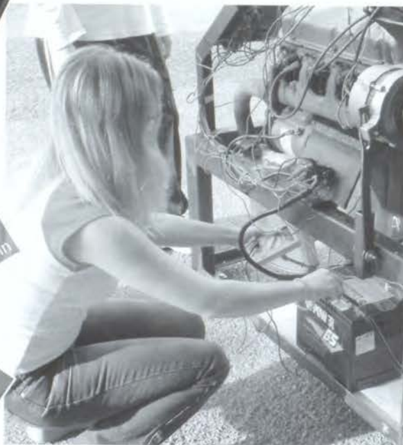
Cranking it up, sophomore Joanna Jasin checks the cranking voltage of a battery. This was one mechanical technique Clark taught his Automotive Technology students during the year.
