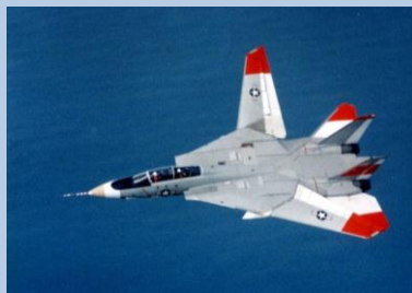
Grumman F-14 Tomcat FF: December 21, 1970 (USA) I: Sept 1974 P: 1969-1991 M: 4 B: 712 S: In service by Iran A.F.
