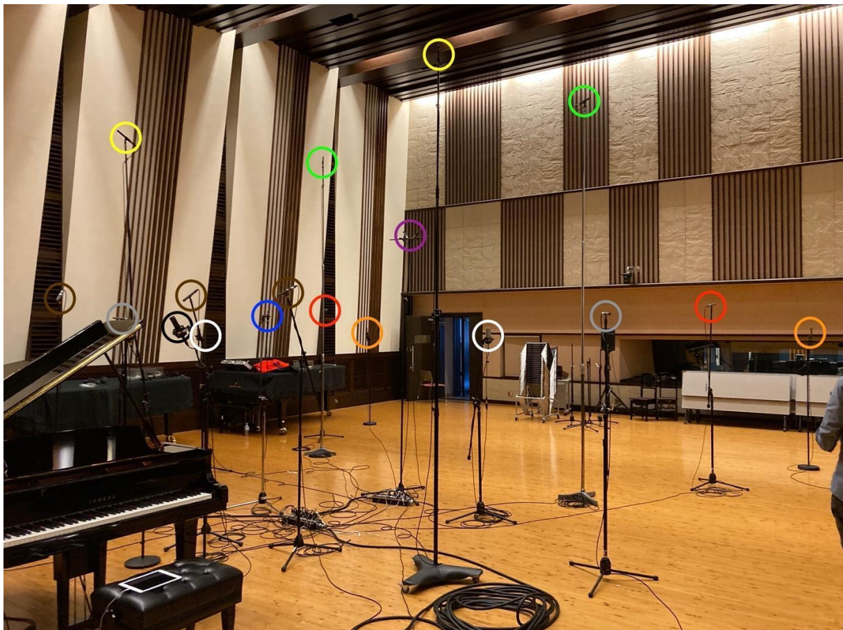
Figure 3. Piano microphone placement, view from the north end (upstage right)
