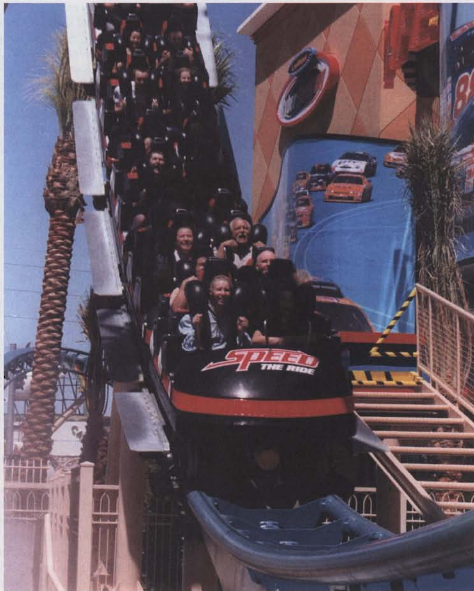
Defying gravity: The Vegas Strip's SPEED—The Ride (above), is powered by linear induction motors, instead of gears and pulleys. An artist's rendering of Premier Rides's planned 500-foot Ferris wheel (right), complete with luxury cabins and a restaurant.
