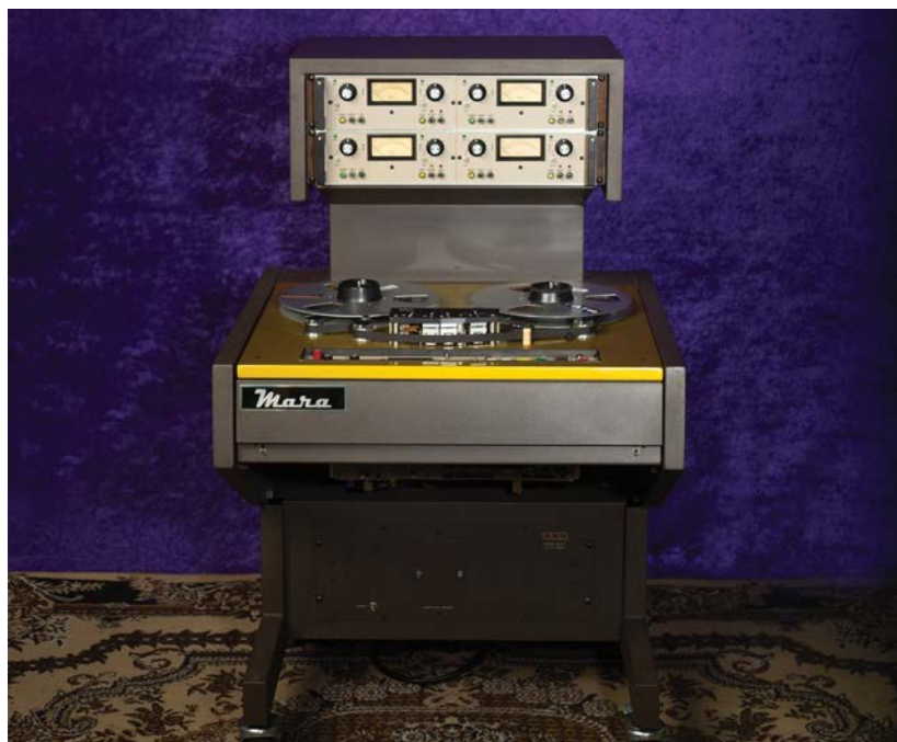
A restored Mara Machines MCI JH110 1/4" recorder includes relapped sync and erase heads with a new repro head, a repainted deck and XLR I/O.
