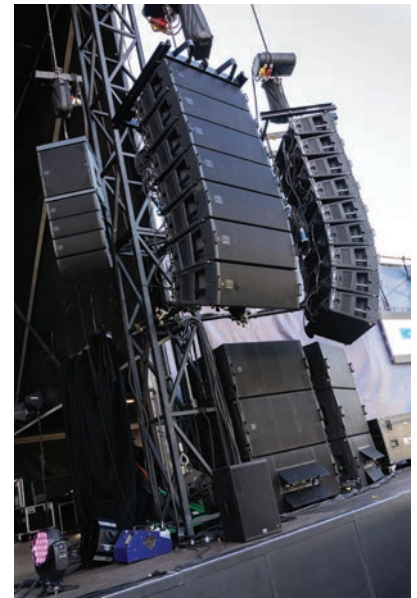
The Martin Audio MLA Compact P.A. is played wide at the Henley Festival's Floating Stage in order to cover the shallow but wide audience area.
