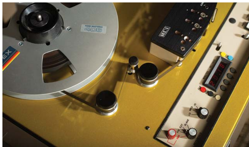
The recorder stores alignments for all speeds and makes it easy to toggle between 7.5, 15 and 30 IPS so the user can compare the differences before committing to a favorite speed.
