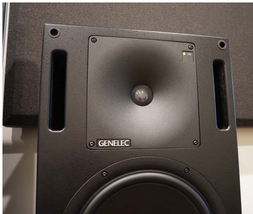
The Genelec 1032C features an active digital crossover that splits the signal feeding the 1-inch metal dome tweeter and 10-inch woofer, both of which are powered by onboard Class D amplifiers.
