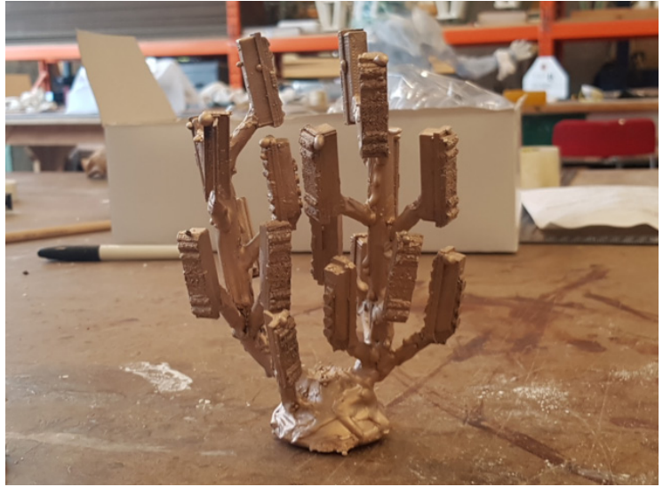
Fig. 10. The structure in Figure 7 after it has been used in the burnout. Both the plastic and wax have been replaced by metal, but still retain their original textures. The gating will have to be manually removed. Image by author
