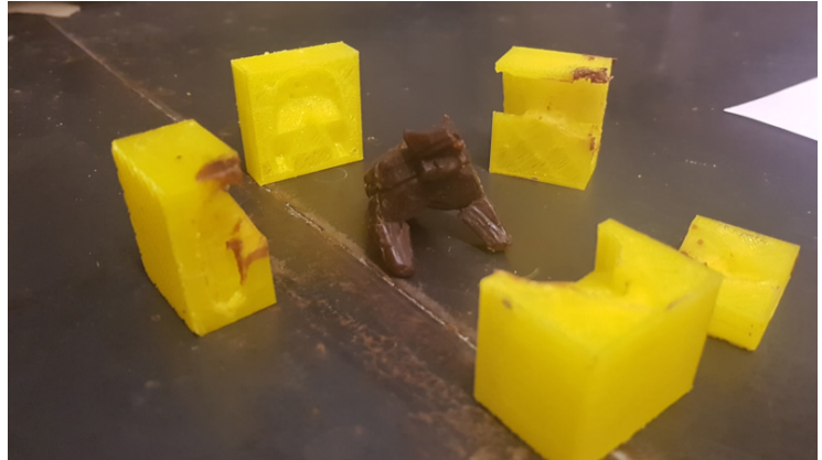
Fig. 3. The components of a 3D printed mould, and the closest thing to a full wax rendering of the desired object achieved by this method placed in the center. Image by author.
