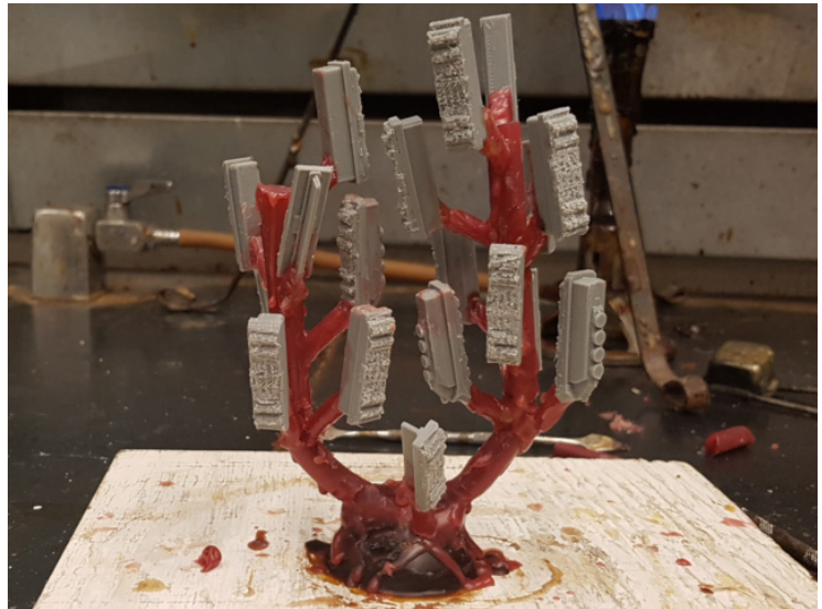
Fig. 9. Several 3D printed components in preparation to be burnt out. They are connected with wax to a central point where the liquid metal will be poured. Image by author.
