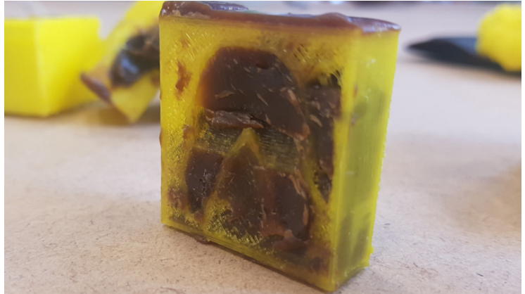
Fig. 4. The remnants of a 3D printed mould that hot wax was poured into. On the right of the image, it is possible to see where an interior cavity of the 3D printed mould was filled with wax. Image by author.
