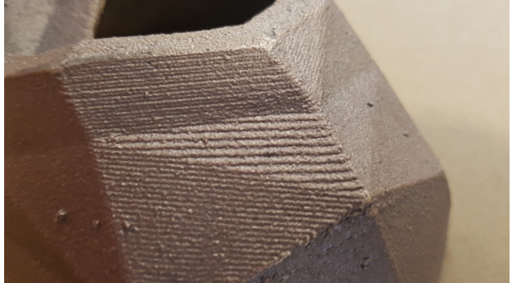
Fig. 7. A bronze version of the object in Figure 4. While the detail left by the 3D printing process can still be seen, nodules of metal can be seen on the surface, caused by the irregular surface of the plastic original. Image by author.
