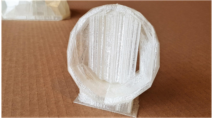
Fig. 1. (a) The supports required to print an overhanging object. (b) A 3D printed object smoothed with a heat gun. The heat warped the plastic to show the structure inside the object. (c) The aftermath of a failed print. Images by author.
