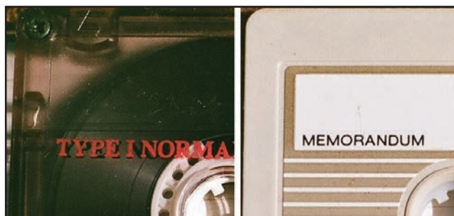
Figure 1: Cassette shells held together with screws (left) are much easier to work with than shells held together with glue (right).
