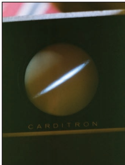
Figure 2: These oscilloscope patterns show the results of azimuth adjustment. The left channel signal controls one axis of the display, the right channel controls the other. When played back in mono, you would ideally see a perfectly straight, thin diagonal line; any bulging indicates that the azimuth is off. On the left is a tape with azimuth out of whack; on the right is a tape with azimuth almost perfect. If you don't have a scope, listen for high frequency response and trust your ears.
