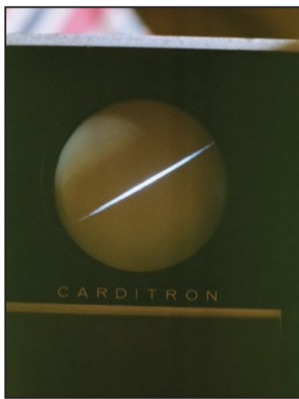
Figure 2: These oscilloscope patterns show the results of azimuth adjustment. The left channel signal controls one axis of the display, the right channel controls the other. When played back in mono, you would ideally see a perfectly straight, thin diagonal line; any bulging indicates that the azimuth is off. On the left is a tape with azimuth out of whack; on the right is a tape with azimuth almost perfect. If you don't have a scope, listen for high frequency response and trust your ears.
