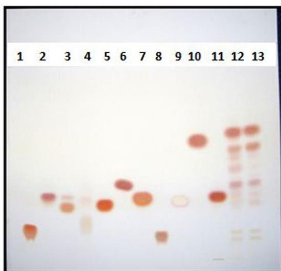
(B) Thin layer chromatogram of total free amino acids. 1-11 Standard amino acids, 12- Forest sample, 13- Domestic sample
